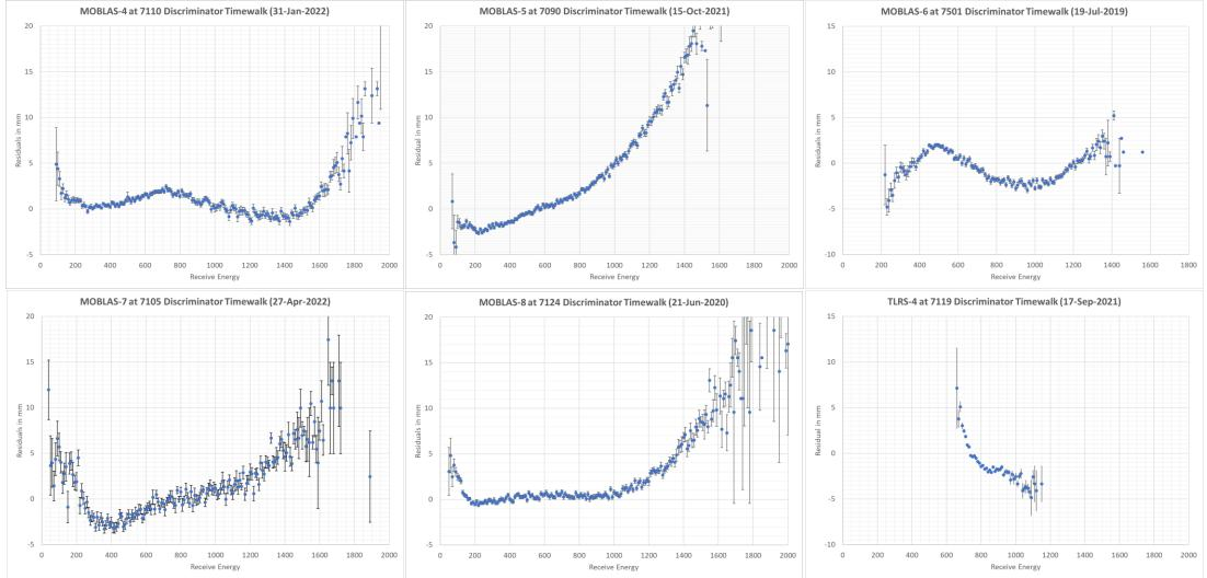
The NASA SLR systems employ two cascading discriminators to minimize timewalk in its Constant Fraction Discriminators (CFDs).
