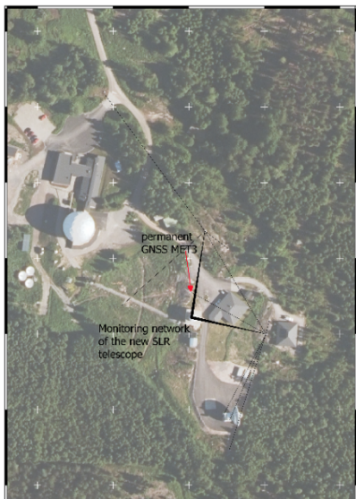
Figure 1. An aerial image of the MGRS showing the measurements from the pillars to the SLR and reference pillars.
