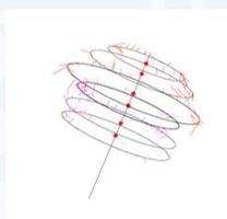
Figure 2. Circle fit. Eight circles with the common axis have been fitted to the coordinates of tracked prisms
