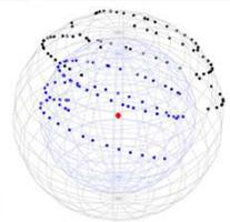
Figure 1. Sphere fit. Two spheres with the same centre have been fitted to the coordinates of tracked prisms
