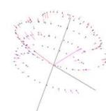
Figure 3. Antenna model. Reference point coordinates, azimuth axis, elevation axis, offset of axes and vectors to the points in zero position have been fitted to the coordinates of tracked prisms
