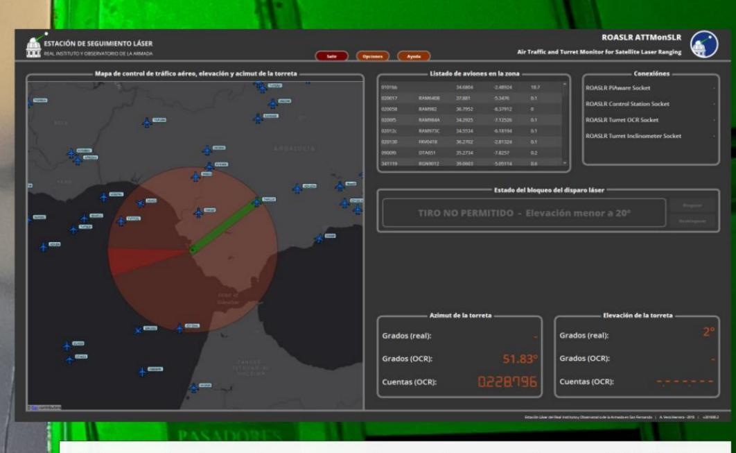
Air safety alert system based on ADS-B
