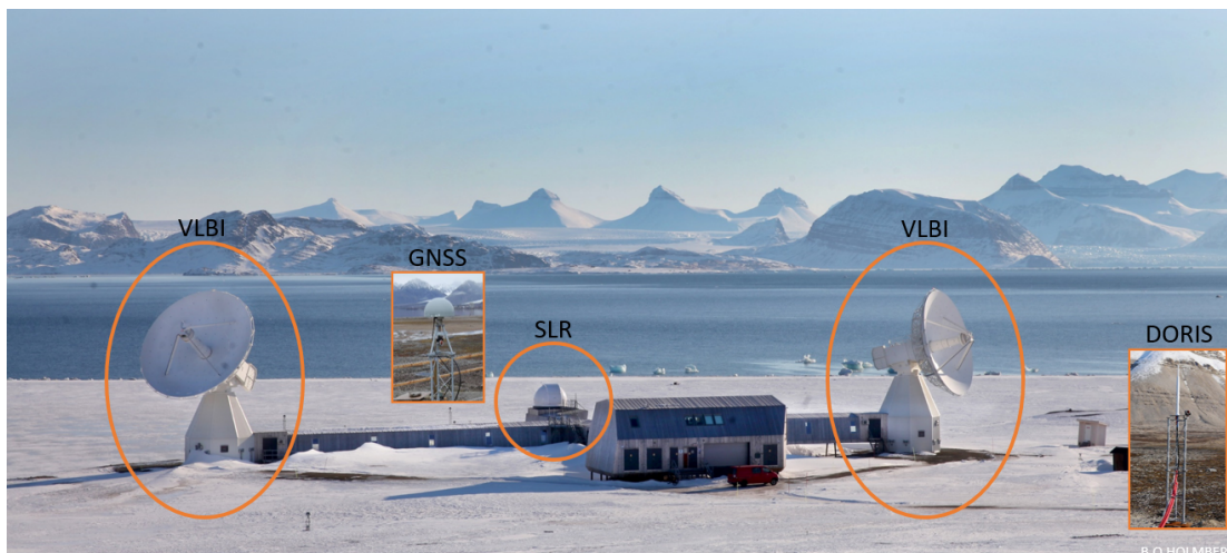
Figure 2. When the SLR is finished, four space geodetic measurement techniques will be co-located at the Ny-Ålesund geodetic observatory: Two VLBI antennas, GNSS receivers, DORIS ground station and SLR station. Photo: Bjørn-Owe Holmberg
