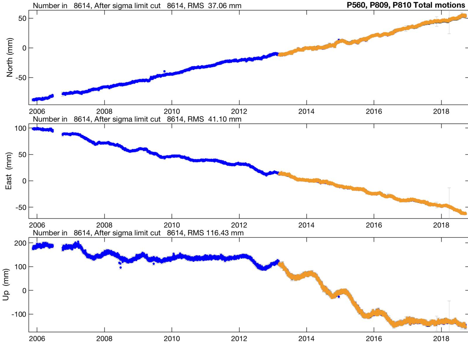
Results for standard UNAVCO GAGE project processing. These are available on web. Large motions are due to tectonics and ground water removal
