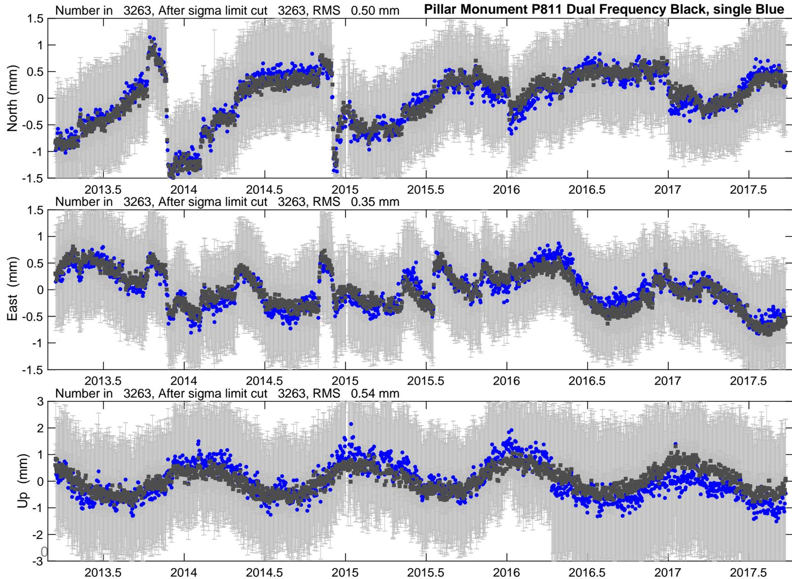
Pillar is unstable at 1 mm level; physical motion implied similar L1+L2 and LC changes. Rapid change at times of rain.
