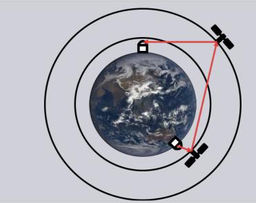
Figure 8: Principle of Ground-Satellite, Satellite-Satellite, and Satellite-Ground Laser Communications
