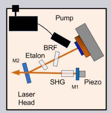
Figure 1: Semiconductor Guidestar Laser Cavity Layout (Credit: Areté Associates)
