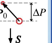
where  $P_0$  is the relative vector from the large CCR to the small one, **S** is the unit vector to the observation station.
