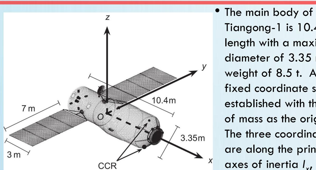
Tiangong-1 is 10.4 m in length with a maximum diameter of 3.35 m and a weight of 8.5 t. A bodyfixed coordinate system is established with the center of mass as the origin O. The three coordinate axes are along the principal axes of inertia  $l_x$ ,  $l_y$ ,  $l_z$ .
