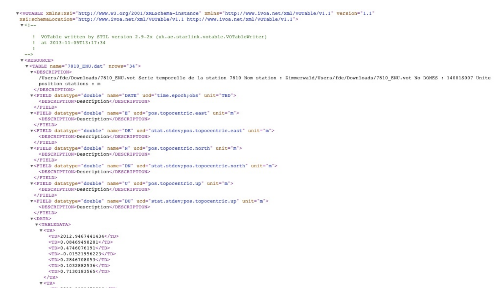
Figure 6: Space Station Coordinates time series (Zimmerwald), provided through the VOTable format. Such files can easily and automatically be built thanks to dedicated tools from common ASCII files, such as "stlits" and "TOPcat".
