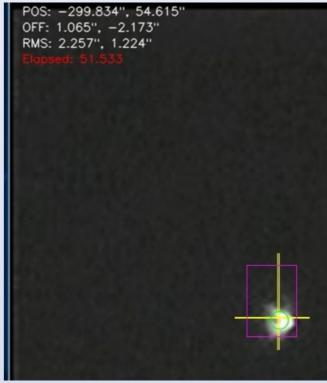
Software, shown here on the left, has been developed to analyze video of star and satellite tracks to measure movement throughout the FOV of the test cameras. The image software will compute statistics of the star/satellite movement including X & Y min/max, mean, and RMS values. This data will help to verify the SGSLR GTA pointing capability.
