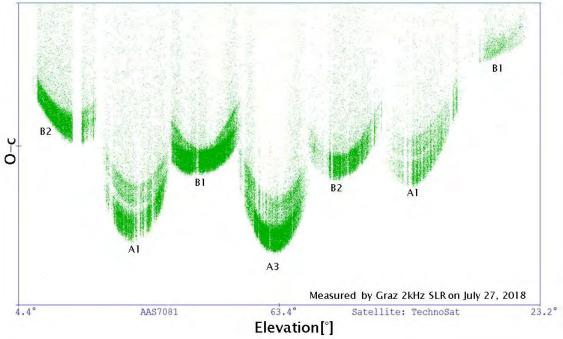
Figure 8: TechnoSat spin in the sequential order of B2  $\rightarrow$  A1  $\rightarrow$  B1  $\rightarrow$  A3 $\rightarrow$  B 2  $\rightarrow$  A1  $\rightarrow$  B1
