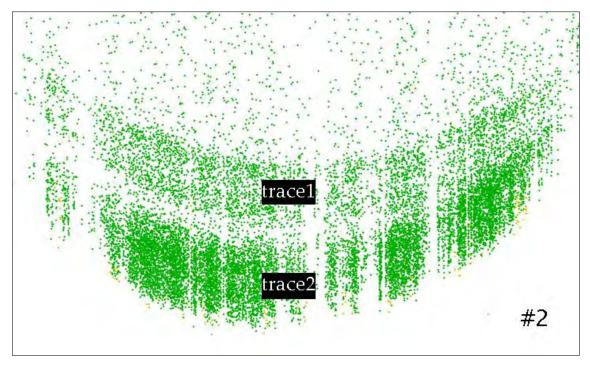
Figure 6: Two traces of laser returns, where the RMS and signal density of trace1 are less than of trace2
