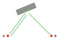
Fig. 1 laser time transfer between two stations by diffuse reflections from a rocket body. Each station performs two-way ranging to the rocket body. In addition to that, each station performs one-way detection of the laser pulses from the respective other stations. That is: 1 shot fired per station and 2 returns detected.
