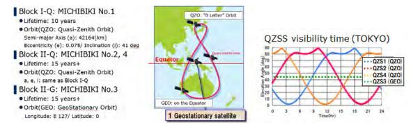
Fig. 1 Orbital elements and orbit of QZSS.
