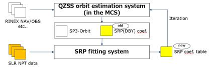
Fig.5 the determination flow of SRP coefficients
