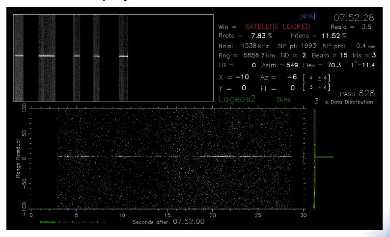
Current points in the NP are shown, along with approximate precision. At this point we are set to switch to a GNSS satellite.
