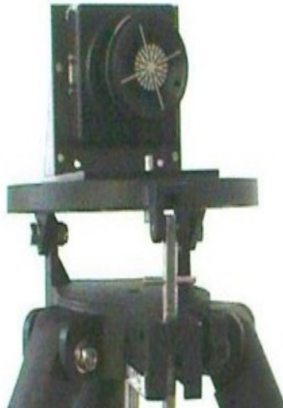
Figure 3: The Single Photon Avalanche Detector package used for Calibration Device on a tripod installed in front of the SLR telescope
