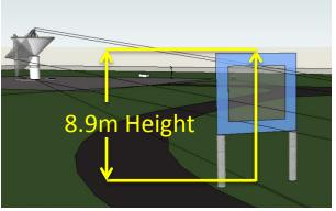
RFI Blocker size takes into consideration full range of motion of VLBI antenna, and distance to SLR radar. Its centerline is located along the Radar-VLBI baseline.
