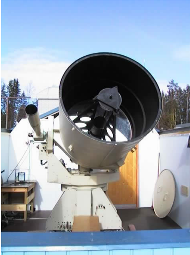
Figure 3. The third generation SLR telescope of FGI with 1m main mirror. Photo: FGI
