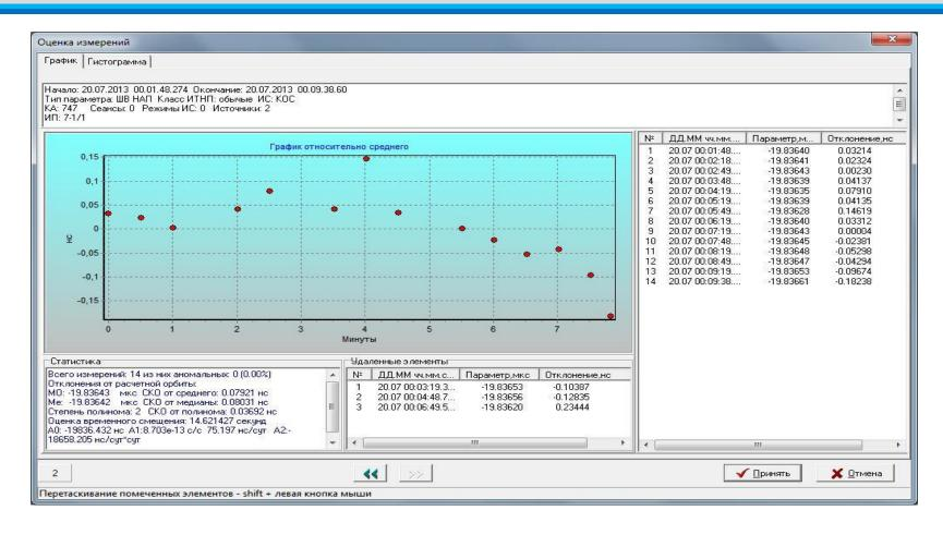
The error (RMS of 2<sup>nd</sup> degree polynomial) of comparison of the S/C onboard clock with reference frequency standard of ground one-way SLR of Altay Laser Center is 37 ps.
