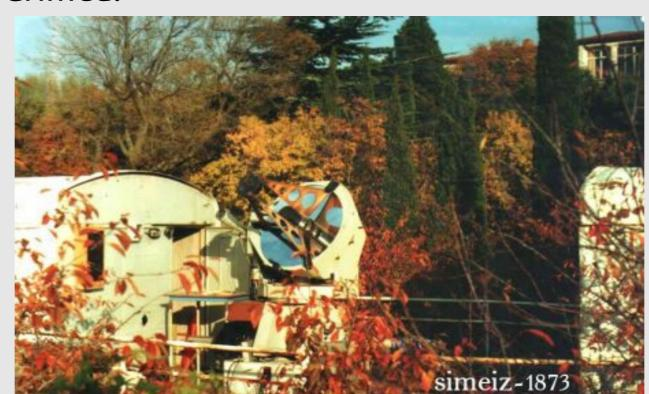
Laser Nd:YAG, 532 nm, 3-10 Hz, 30 - 80 mJ Telescope TPL-1M, coude focus, 1 m, Expected overall accuracy of the system is 2 cm Active work from 1988. Statistics of observations, normal points from 01.01.2013 [3]: LEO - 1042 LAGEOS - 178 HEO - 26
