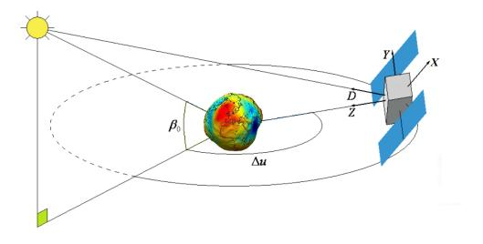
**Figure 2.** Sun fixed reference frame for dynamical orbit parameters of GNSS satellites (Beutler et al., 1994). GNSS dynamic orbit parameters estimated in standard CODE solutions read as follows:  $D = D_0$ ;  $Y = Y_0$ ;  $X = X_0 + X_S \sin \Delta u + X_C \cos \Delta u$ .
