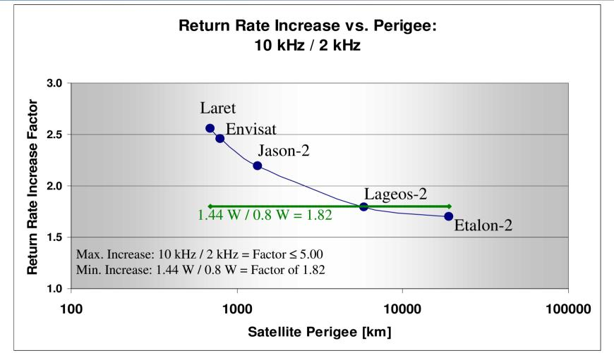
1.44 W @ 10 kHz / 0.8 W @ 2 kHz = 1.82; for Single Photons, we will arrive at this ratio; For Single Photon Satellites (HEOs and LAGEOS): Theoretical Factor 1.82 expected; For Multi –Photon Satellites (LEOs): The Factor will increase, according to received energy (distance ...)
