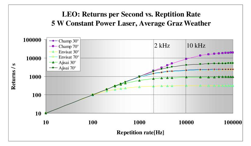
Assumed: 5 W Constant Power Laser / C-SPAD / Graz Atmosphere: LEO: Significant increase of returns / s at least until 10 kHz
