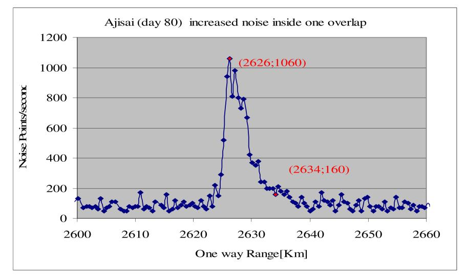
During OVERLAP: Noise increases from 100 Hz to 1 kHz ☺ (Overlap Avoidance switched OFF)
