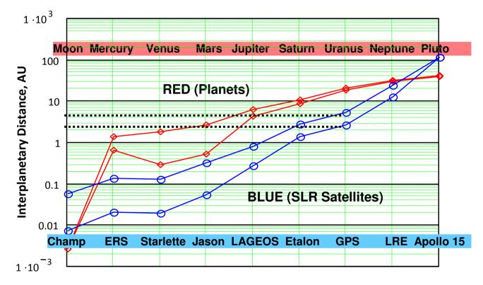
Red curves bound the Earth-planetary distance (1AU ~150 million km) Blue curves bound the equivalent transponder range at satellite elevations of 90 and 20 degrees respectively.
