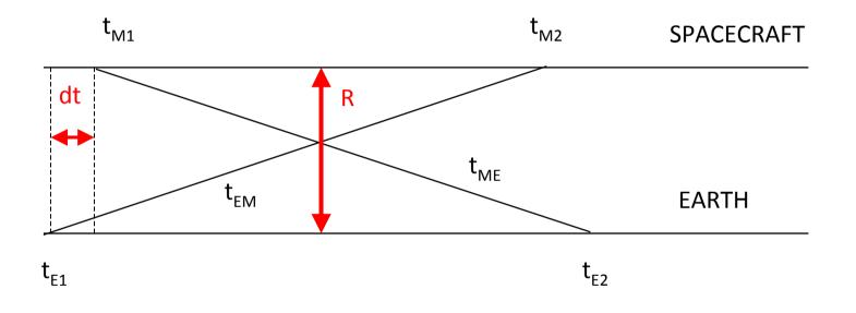
Range  $R = c(t_{ME} + t_{EM})/2 = c[(t_{E2} - t_{E1}) + (t_{M2} - t_{M1})]/2$
