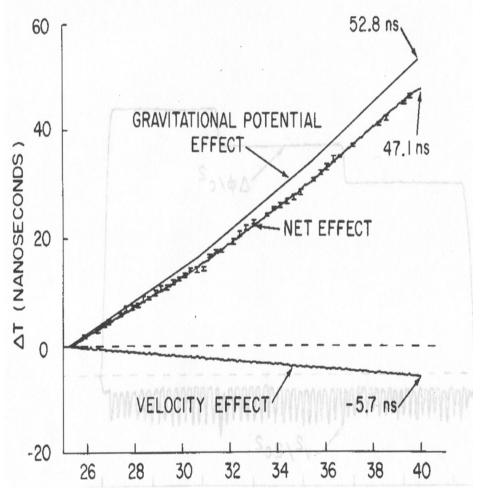
Transponders can sense the localized gravity field via its effect on an atomic clock. Average drift rate was 3 nsec/hr or 50 psec/min or 0.8 psec/sec or less than one part per trillion!
