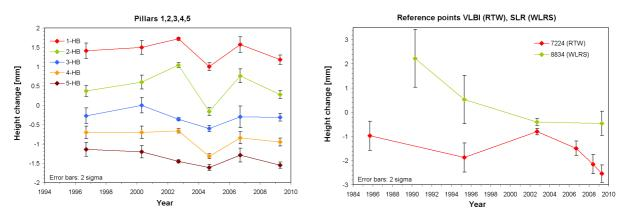
Figure 2: Height variations of survey pillars (left) and reference points of the VLBI and SLR system (right).
