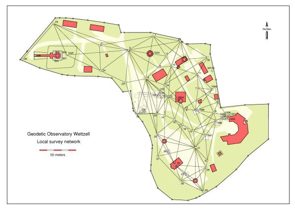
Figure 1: Local survey network at the Geodetic Observatory Wettzell.
