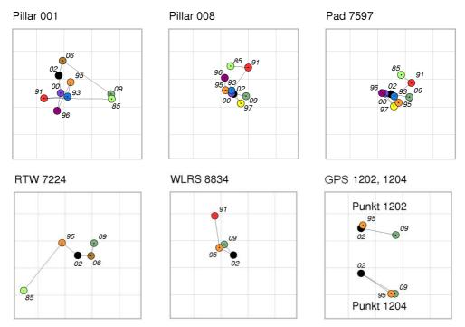
Figure 3: Horizontal motion of selected survey marks (top) and reference points (bottom). Line spacing is 1 mm, years are indicated by numbers.
