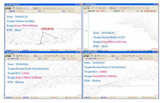
Figure 7 some results of un-cooperative target laser ranging
