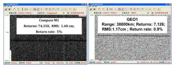
Figure 3 kHz repetition rate SLR measuring results
