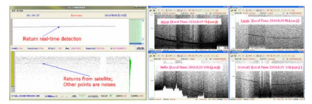
Figure 4 Daylight SLR measuring results for LEO satellites
