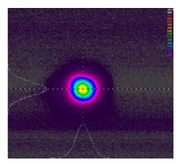
Figure 2. The figure of the RG laser Mode Profile: the laser beam quality M2 factor is 1.11
