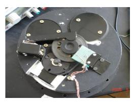
Fig. 1 The machine frame of the adjustable iris
