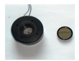
Fig.2: Spectrum filter in constant temperature box
