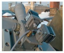
Figure 2: Collimator and alignment motors
