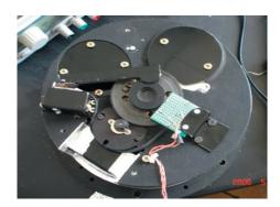
Fig. 1: The machine frame of the adjustable iris
