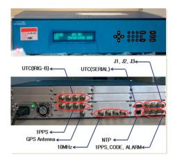
Figure 2: Front panel(upper) & rear panel(lower) of timing system(XII, SYMME-TRICOM INC. 2008) installed in KASI
