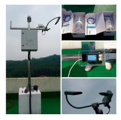
Figure 3: Pre-installed weather monitoring system in KASI: Total weather transmitter (WXT520), Rain detector (DRD11A), Visibility sensor (PWD52)
