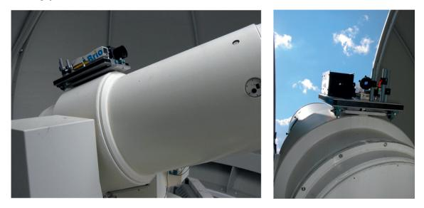
Figure 1: The auxiliary ranging system on top of the telescope of the WLRS.
