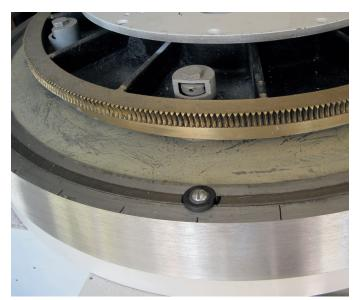
Figure 3: The azimuth rail. Black marks on the circle show the levelled points on the rail. The rod was placed on the magnet button to reduce error due to placing of the rod on the rail.
