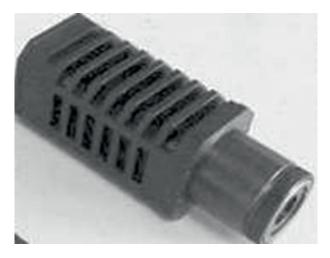
Figure 5: The SPAD detector package optimized for kHz single photon only ranging purposes.
