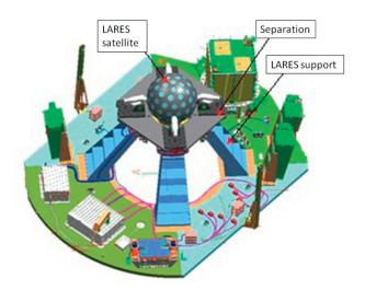
Figure 2: LARES System. Image taken from reference "Objectives of LARES Satellite".
