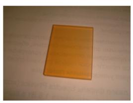
Fig. 4: Holographic selector recorded in PTRG
