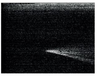
Fig.5. 200 times exposure modulation, exposure time 67  $\mu\text{s}$
