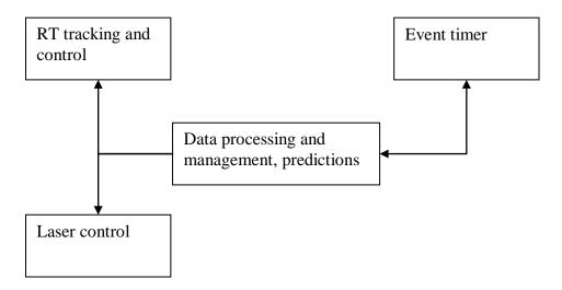
Figure 1. Software organization at SLR station Riga
