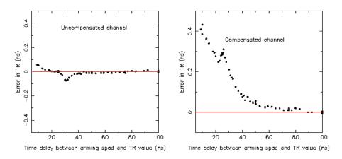
Figures 1 and 2. Range bias variation of the uncompensated and compensated C-SPAD channels with time of observation after gating.
