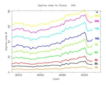
**Figure 3.** The percentage of lost observation opportunities due to daytime noise detection during a Champ pass during the first 10, 20, 30, 50, 75, 100, 150, 200 and 250 nanoseconds after the gating of the C-SPAD.
