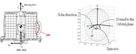
Figure 4. Mounted Position of LRA
