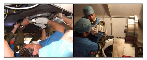
**Figure 4.** Access to the prisms required working underneath the mechanical structure supporting the telescope. Great care was taken to prevent dust from entering the open Coudé path.
