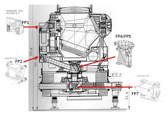
Figure 2. Cross section of the TIGO SLR telescope. The positions of the replaced prisms and their mounts are indicated.
