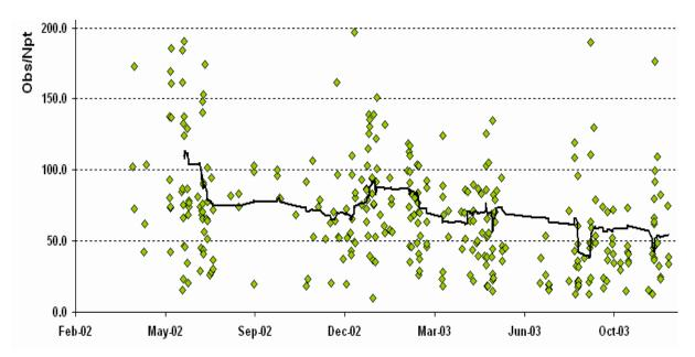
**Figure 1.** Number of observations per normal point at 423.5 nm during TIGO's first two years of operation. The return rate has fallen by approx. 50 % in less than two years, presumably due to the degradation of optical components.
