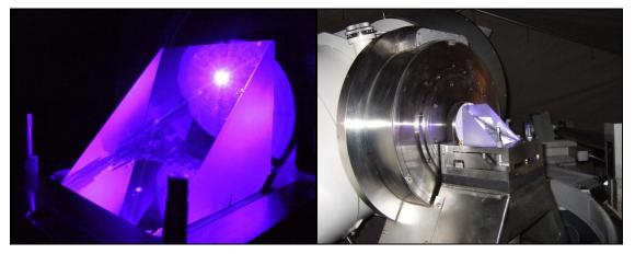
**Figure 5.** The blue (423.5 nm) second harmonic of the transmitted beam was used to realign the optics, utilizing various improvised alignment tools.
