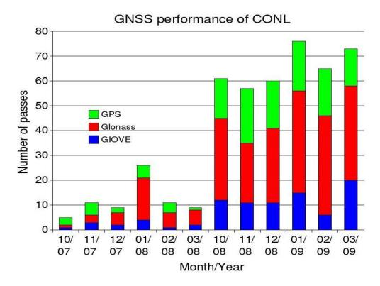
**Figure 6.** GNSS observation statistics for CONL: 6 month of data after the maintenance are plotted (Sept. 2008-March 2009) along with the corresponding period of the previous year. The strong increase of HEO passes per month is a result of the improved system transmission after the telescope upgrade.
