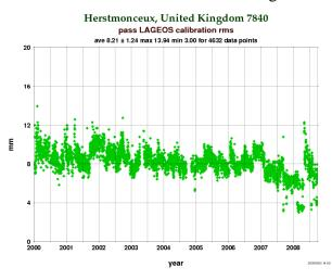
from the ILRS website and shown left. There is a clear drop in RMS at the beginning of 2007 on the installation of the event timer. A further drop in RMS is present for later passes, indicating kHz observations. The later higher RMS passes are due to the temporary use of an older SPAD detector.
