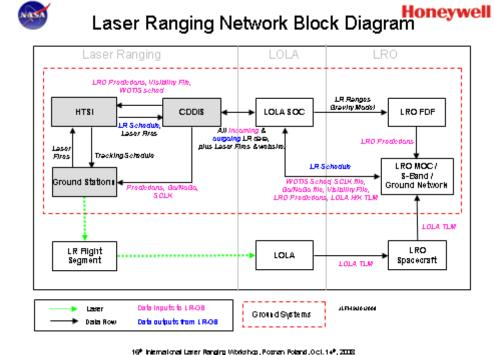
Figure 1. LR-LRO Laser Ranging Network Diagram
