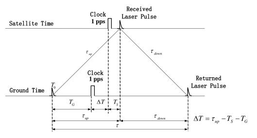
Figure 8. The principle of Laser Time Transfer, where:
