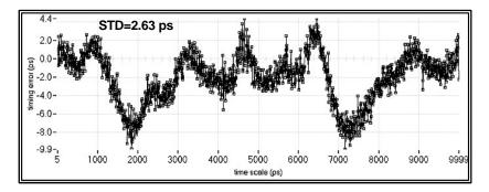
Figure 3. Integral non-linearity over internal clock period 10 ns
