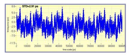
Figure 2. Integral non-linearity over input frequency period 100 ns
