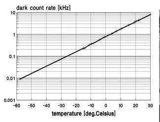
**Figure 3.** The detector dark count rate as a function of chip temperature, SPAD 25 um in diameter biased 0.7 V above, the slope corresponds to a drop of dark count rate of one decade per 30 K.
