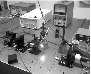
**Figure 4.** The TCSPC experimental setup. Left to right: laser diode, collimating optics, neutral density filters stack, tungsten bulb, SPAD detector holder on X-Y-Z stage. The tungsten bulb (bright in the middle) is used to generate
