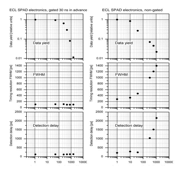
**Figure 5 (left)**. The results summary of TCSPC experiments, SPAD gated 30 ns before arrival of photon of interest, data yield (up), timing resolution r.m.s. and detection delay (bottom) versus background photon flux intensity in millions per second hitting the detector active area.
