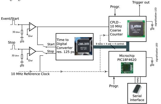
Figure 1. The block diagram of the timing unit
