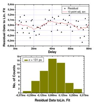
**Figure 5.** The first graph shows the residual data to linear fit, the adjacent averaging over 10 points was applied. The second graph illustrates the histogram of residual data, with standard deviation of 131 picoseconds.
