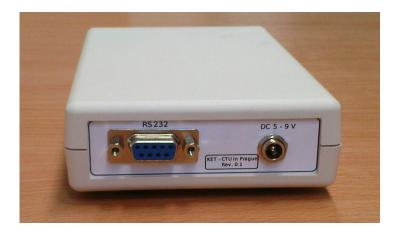
Figure 3. The back panel of the timing unit.
