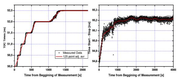
**Figure 6.** The first graph shows the warm up characteristics of the timing unit in event timing regime. Each point represents average of 255 samples. The second graph shows the warm up characteristics of timing unit in start - stop regime. Each point represents average of 255 samples.
