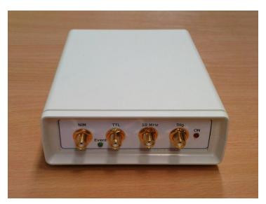
Figure 2. The front panel of the timing unit.
