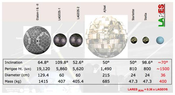
Figure 3. The currently available geodetic targets augmented with the soon-to-be-launched LARES spacecraft.
