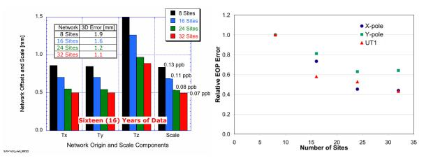
**Figure 6.** Origin and scale accuracy (left) and orientation accuracy (right) as a function of the size of the defining network.
