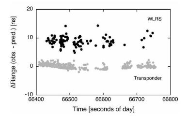
**Figure 9.** The filtered transponder echos from fig. 8. The data recorded on the WLRS exhibits a larger scatter caused by the 3 ns pulse width of the transponder transmitter. The offset between the two tracks is introduced for better visibility.
