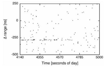
**Figure 12.** Range residual plot of a LAGEOS 1 pass taken on August 19, 2008 using the transponder module alone. The satellite track is very weak as expected from the low signal level calculated for this case (tab. 1).
