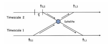
**Figure 3.** Functional diagram of the transponder simulation application. Time is progressing along the x-axis, while the distance is corresponds to the y-axis. For an interplanetary link laser pulses are transmitted directly between the two ranging terminals. In a ground based simulation experiment, geodetic satellites are used to backreflect the laser pulses, so that they can be detected by an independent ranging system on the ground near the transmitting station.
