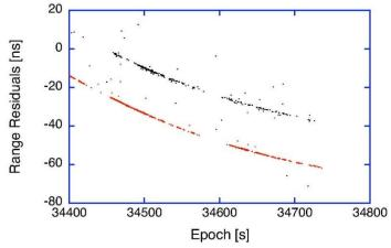
**Figure 2.** Example of a Topex pass observed by the WLRS on June 20, 2001 under cloudy conditions. The returns on the standard ranging configuration are shown on the lower trace, while the echoes on the small extra receive aperture are displayed on the upper trace.
