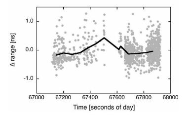
**Figure 11.** Range residual plot of a Beacon C pass taken on August 13, 2008. The residuals are obtained from a linear regression on simultaneous detections on both ranging systems. The black line was derived from this data set by averaging the data over 1 minute intervals.
