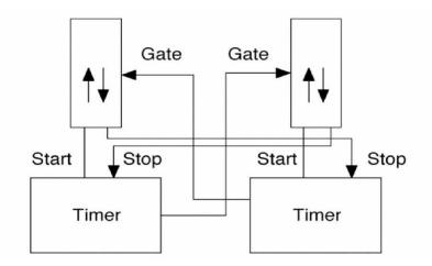
Figure 6. Block diagram illustrating the cable crossover required for the transponder simulation experiment.
