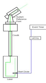
The Transmit-side delay is the sum of the times taken for the laser pulse to travel from the Start Diode to the System Reference Point and the propagation time for the Start Diode electronic pulse to travel through cables and electronic equipment to trigger the Event Timer. Described here are estimates of both these elements.
