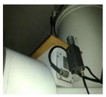
Emitter removed and replaced with flat surface.
