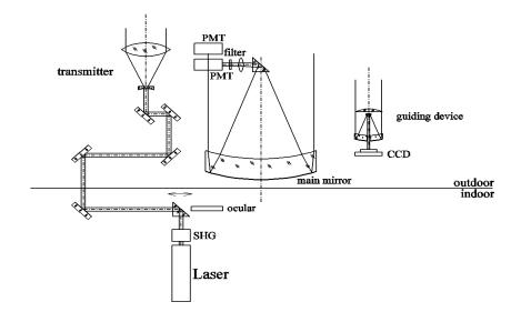
Figure 3. The modified optical scheme
