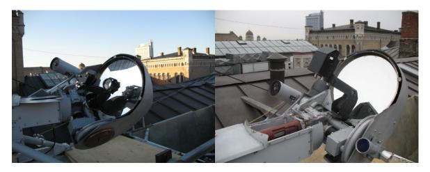
Figure 1. SLR before (left) and after optics modification (right)
