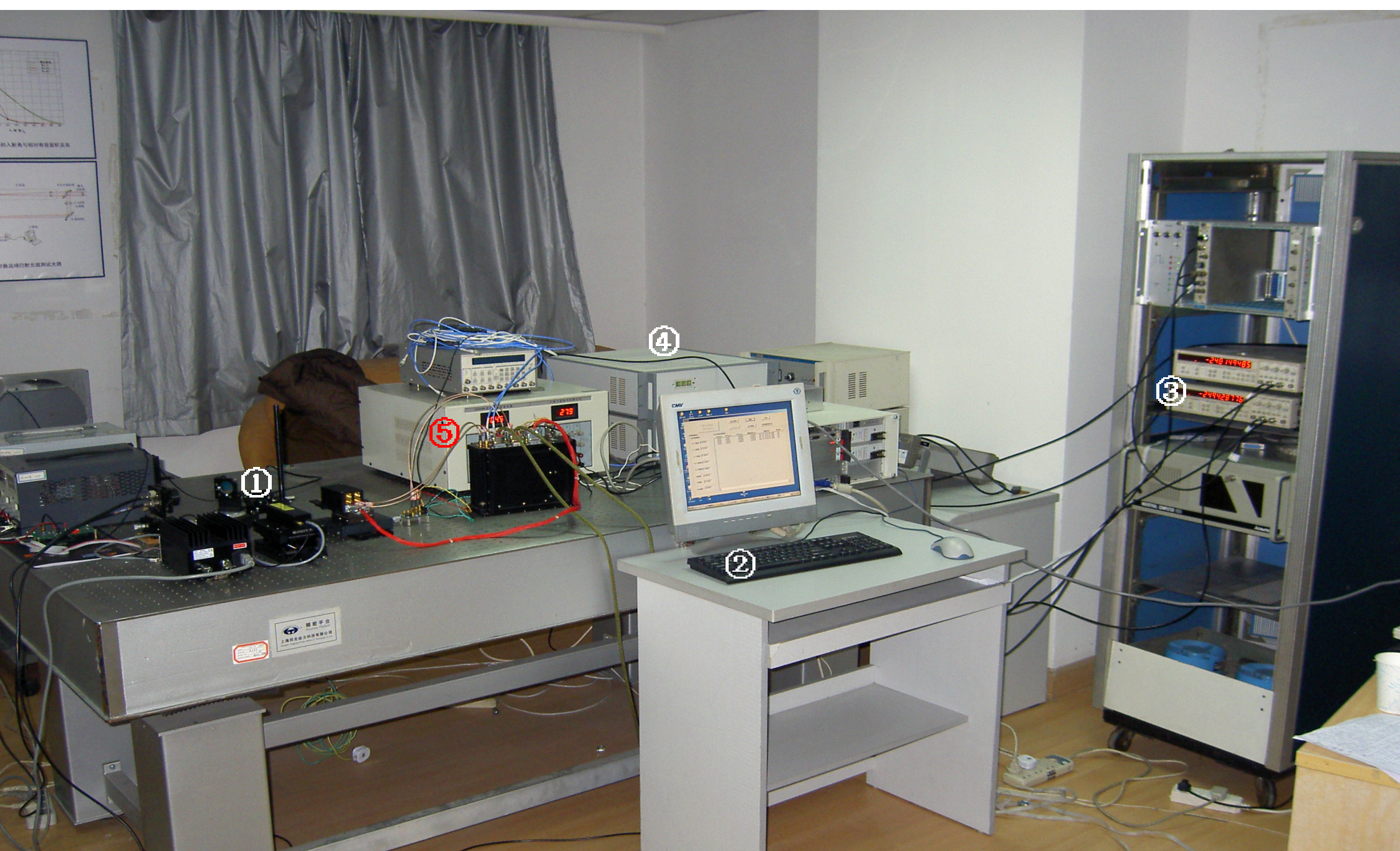
① Optical System ② Computer ③ Counter SR620 (2 sets) ④ Rubidium Standard (2 sets) ⑤ LTT Timer and supply
