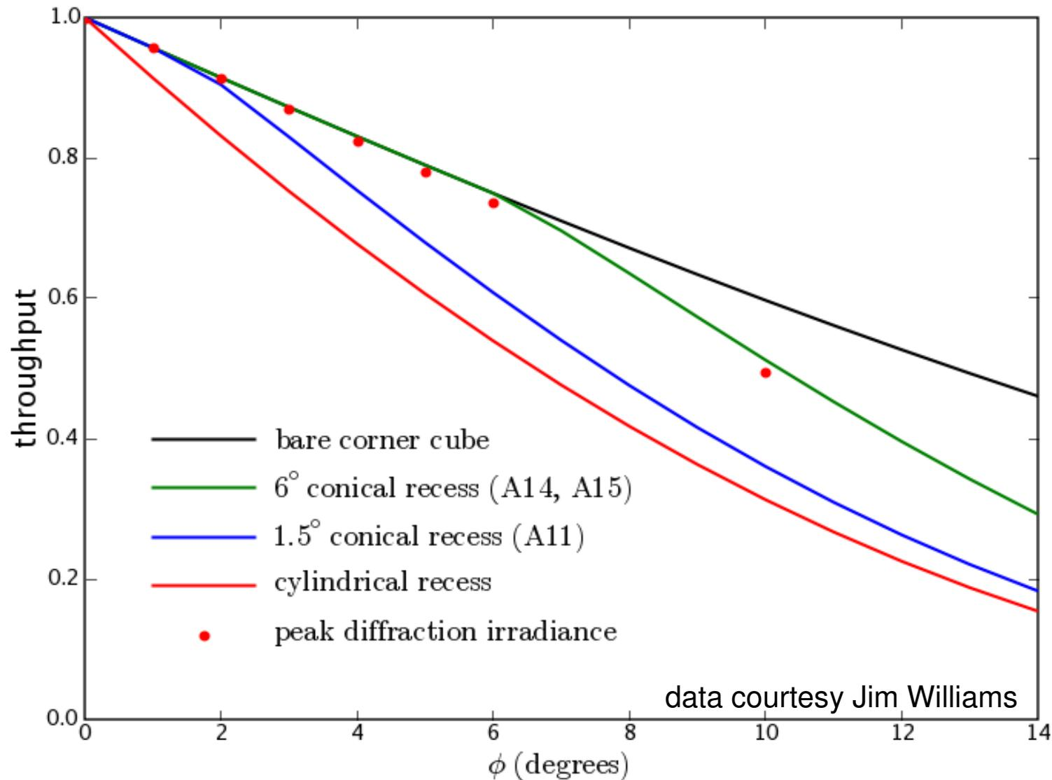
All recesses are half-diameter, and throughput is total geometrical flux. central diffraction irradiance is reduced from this, but not much at first
