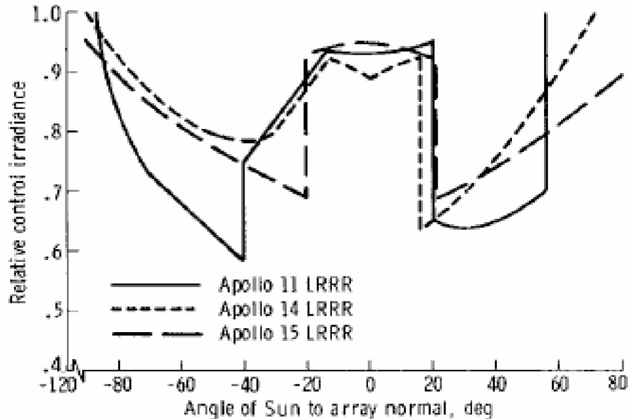
FIGURE 14-4.—Comparison of calculated thermal performance expected from Apollo 11, 14, and 15 LRRR arrays.
