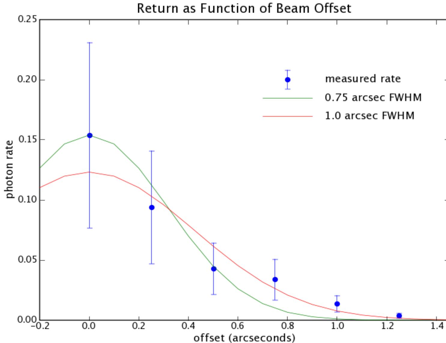
Walking the beam toward optimal signal gives idea of beam profile
