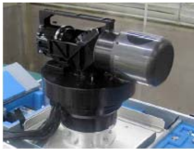
Figure 4: A 10cm class Coarse Pointing Mechanizm (CPM)
