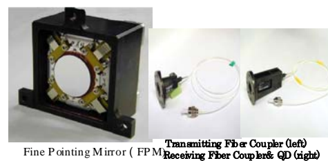
Figure 6: Key components of internal optics
