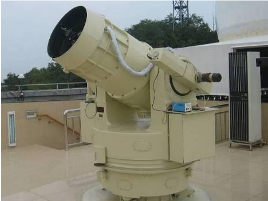
Fig.3. SLR Telescope(Aperture 600mm)
