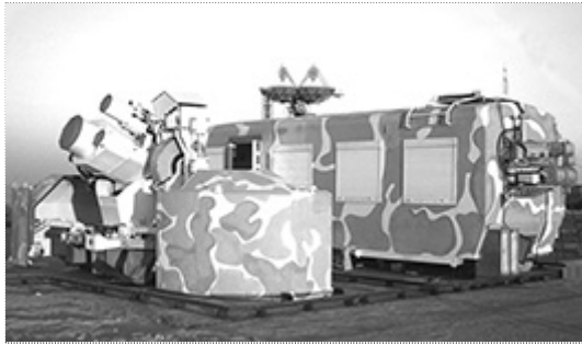
Figure 6: Mobile SLR station installed in Baikonur
