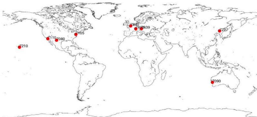
Figure 6. Minimum network used to apply the minimum constraints to define the homogeneous weekly TRFs.
