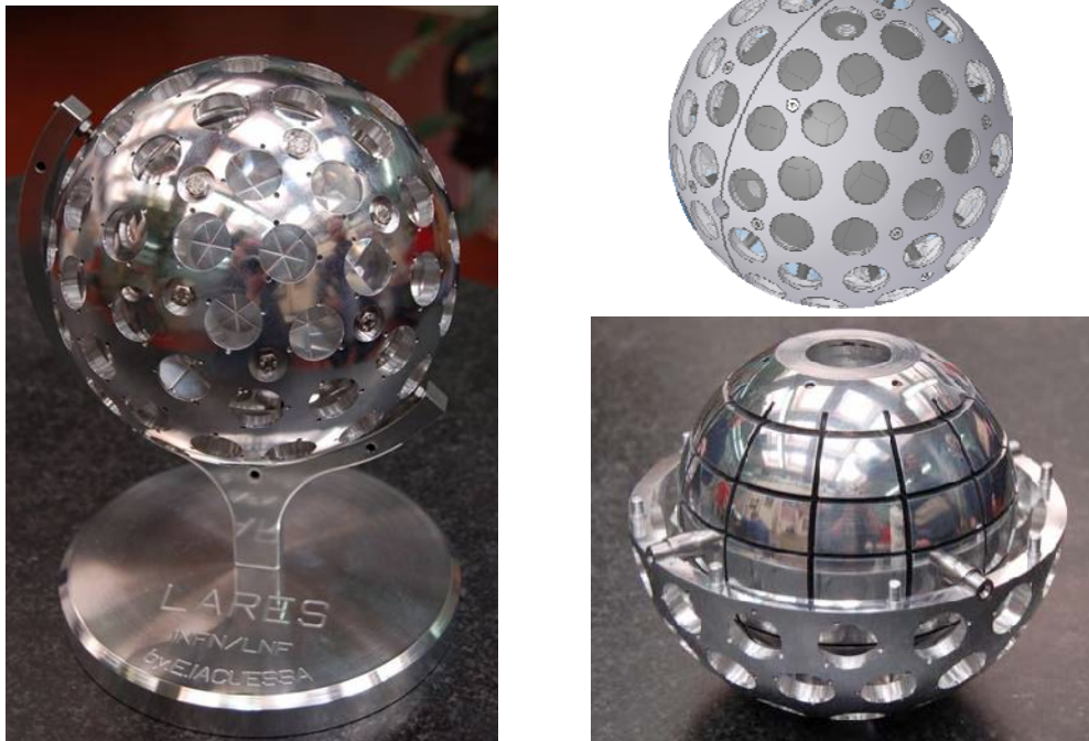
Figure 8. A 1:2 model of the proposed LARES (Bosco et al. , 2006) geodetic satellite for SLR applications in relativistic tests and geodetic TRF development.
