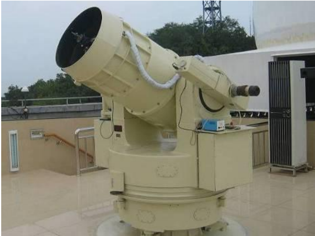
Fig.3. SLR Telescope(Aperture 600mm)
