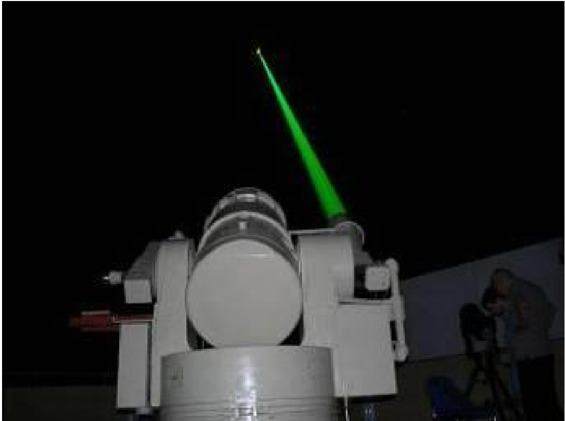
Fig.9. Laser Firing (2J, 20Hz, 40W in 532nm)
