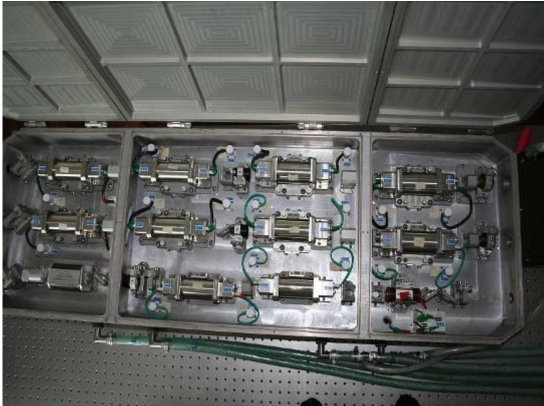
Fig.7. Inside of the 40W Pulsed Nd:YAG Laser
