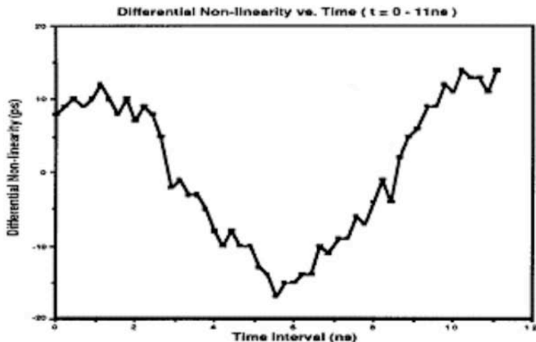
Graph 1: Differential Non-linearity for time differences of 0 to 11 ns. This shows the residual non-linearity of the time-to-amplitude converters.
