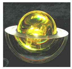
Figure 7. 17 cm-diameter spherical retroreflector (dissembled)
