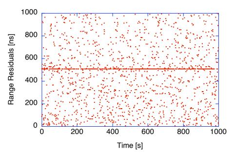
**Figure 5:** Simulated range residuals with a range resolution of 44 cm. The diagram shows an interval of 1000 seconds worth of data computed for a total range of 1600 km with a detection probability of around 20%.
