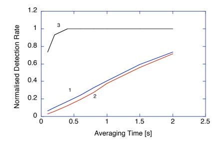
**Figure 4:** Normalized detection rate for the LAPE from an orbit height of 1600 km. A simple return prediction model (1) improves the return rate already noticeably over a plain range-gate evaluation (2). For the case of moderately improved parameters the detection rate improves as in curve (3).
