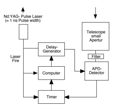
Figure 2: General block diagram of a laser altimeter
