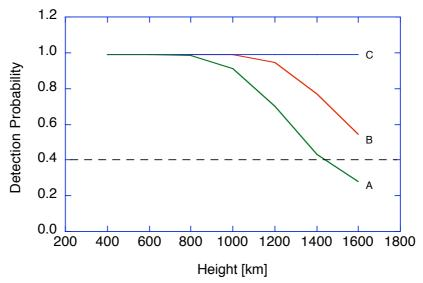
**Figure 7:** Detection Probability versus satellite height of one identified altimeter reading per time bin for 3 different parameter sets similar to table 2. The integration is 1 s and the laser energy was set to 2  $\mu$ J (A), 4  $\mu$ J (B) and 6  $\mu$ J (C).
