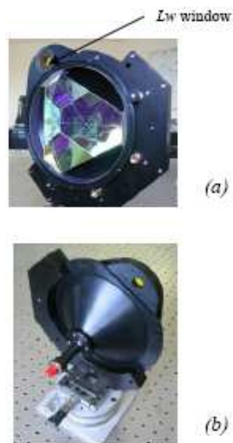
Figure 3 : Prototype (a) front: reflector (b) back: detection optics
