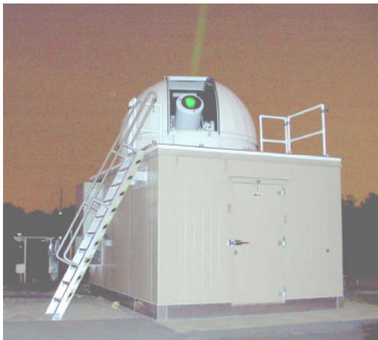
Figure 1: Prototype SLR2000 satellite laser ranging system undergoing field tests at the NASA Goddard Space Flight Center.
