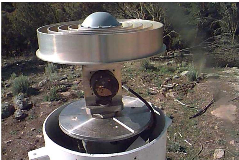
Figure 4: Example of very close collocation, between calibration target retroreflector, GPS antenna and survey monument plate on top of the North pillar.
