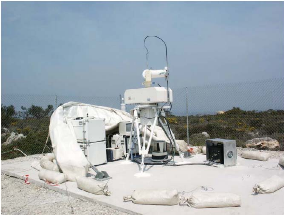
Figure 3. FTLRS deployment at the TUC campus, the ranging system on the pad.
