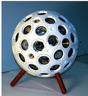
Figure 5. LARETS. Orbit height 690 km. Used for scientific and applied tasks in geodesy and geodynamics
