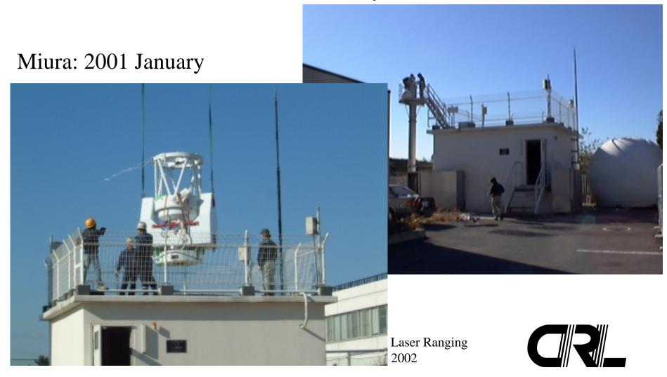
Integration of Keystone Lasers and 1.5m telescope (50mJ/20Hz/50ps high precision setup)
